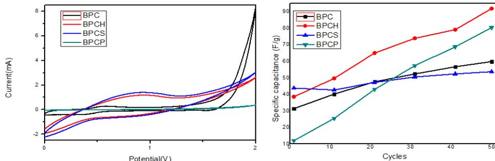
**Fig. 3** (a) CV curves of BPC, BPCH, BPCS and BPCP a scan rate of  $30 \text{ mVs}^{-1}$ , (b) Cycle stability of BPC, BPCH, BPCP and BPCS.
