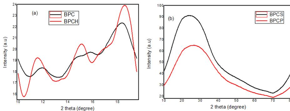
Fig. 1. XRD diffraction patterns of (a) BPC and BPCH (b) BPCS and BPCP.
